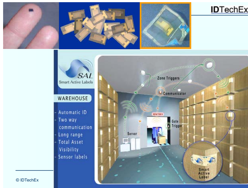
Fig. 5.3 Printed batteries from Infinite Power Solutions and the concept by the Smart Active Labels Consortium of using RFID smart labels with similar batteries to boost range in warehouse environments.
